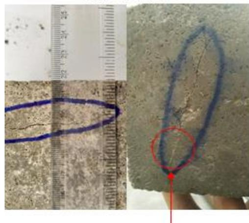
**Fig 4: Cracks formed and Healed**
