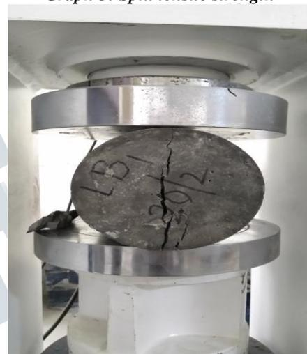
**Fig 3: Split tensile strength testing**
