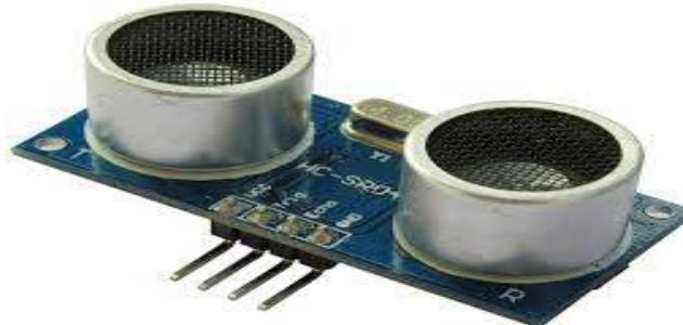
Fig 2 Ultrasonic Sensor
