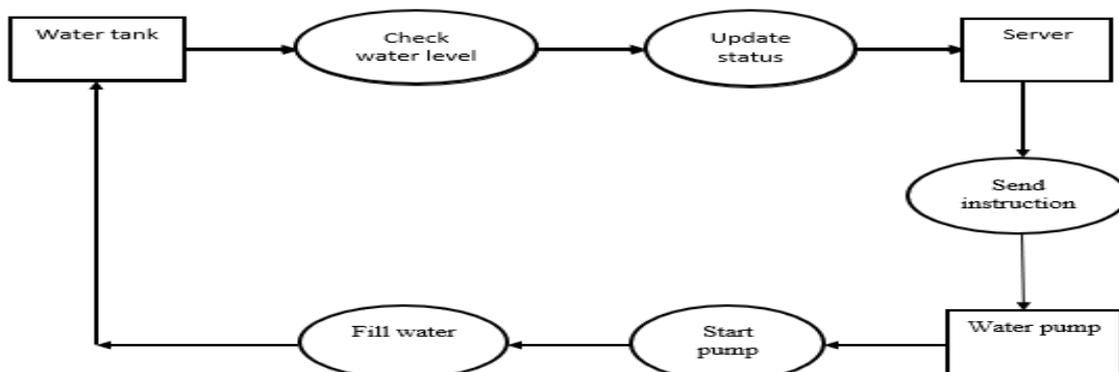
Fig 3 Control System of motor
